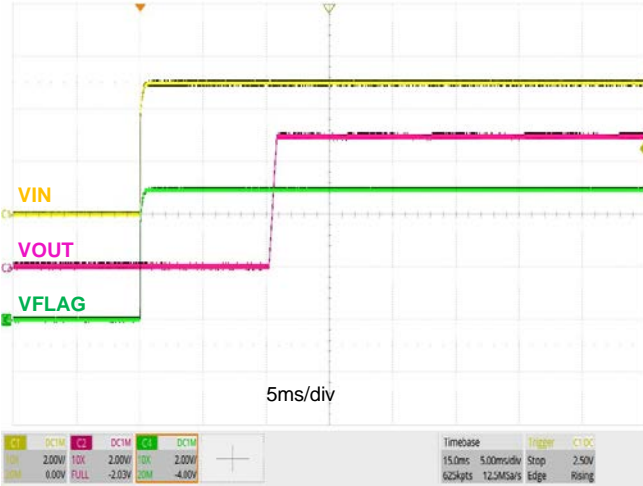
Power on Response (No Load)
