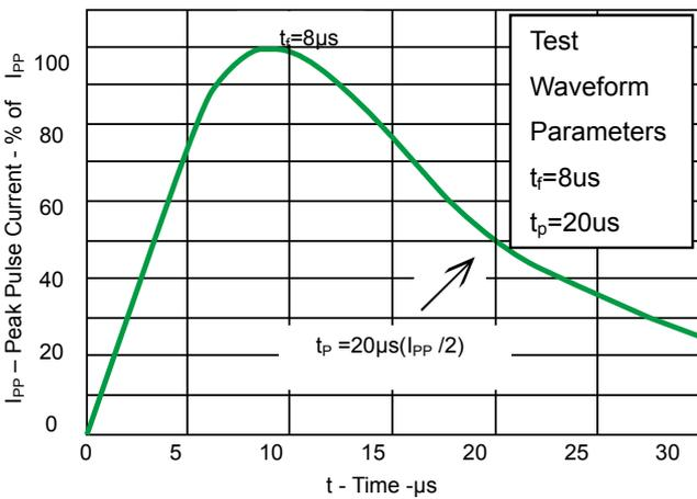
Fig 1.Pulse Waveform
