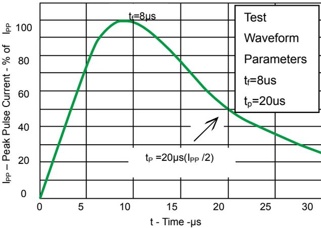
Fig 1.Pulse Waveform
